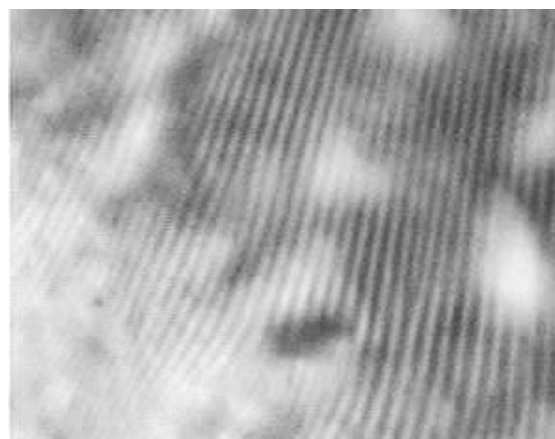
Figure 40. Defect lines of a helical domain in the nematic phase of compounds 49 h (magnification: \times 100 ).
