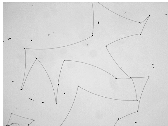
Figure 35. Bowed disclination lines in a TN device containing E7 doped with 0.0027 wt % of CB15, resulting in a pitch of 0.4 mm, (magnification: \times 100 ). The black dots are the spacers which are used to separate the cell surfaces.
